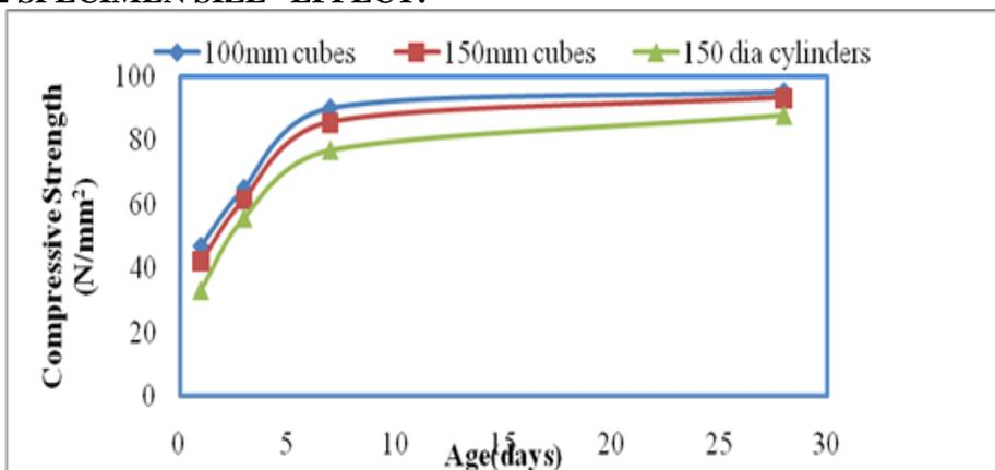
**Fig3.1 Variation showing compressive strengths of 100 mm cubes, 150mm cubes and 150 dia. cylinders with respect to Age(days)**
