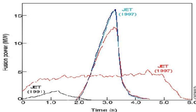
*Figure 1: Fusion energy production in the Joint European Torus (JET) [5].*
